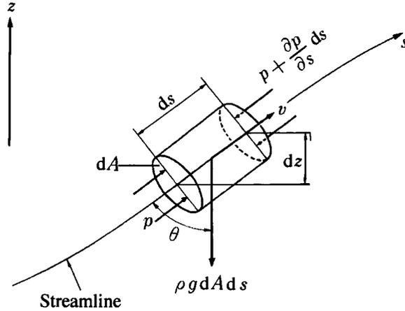
**Fig. 5.4** Force acting on fluid on streamline
