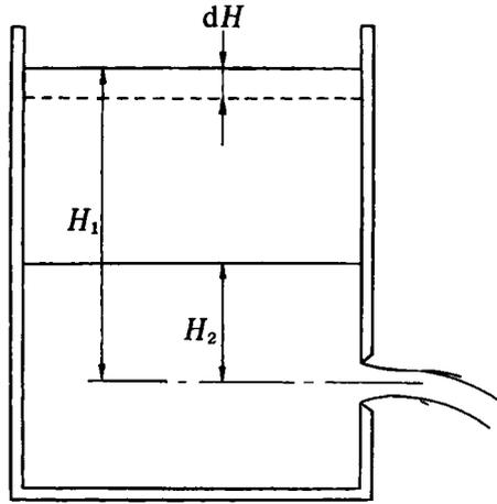
Fig. 5.12 Flow through a small hole (2)
