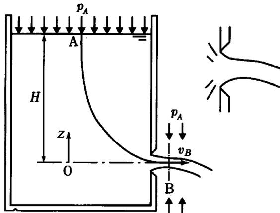
Fig. 5.11 Flow through a small hole (1)
