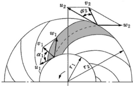
Fig. 5.24 Flow along blade of centrifugal pump
