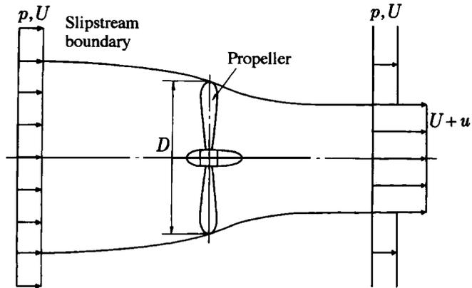
Fig. 5.21 Flows upstream and downstream of a propeller
