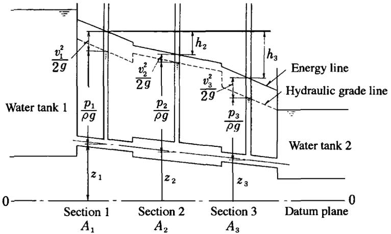
Fig. 5.7 Hydraulic grade line and energy line
