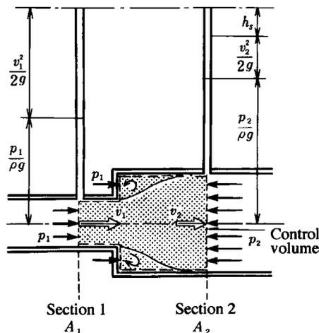
Fig. 5.19 Abruptly enlarging pipe
